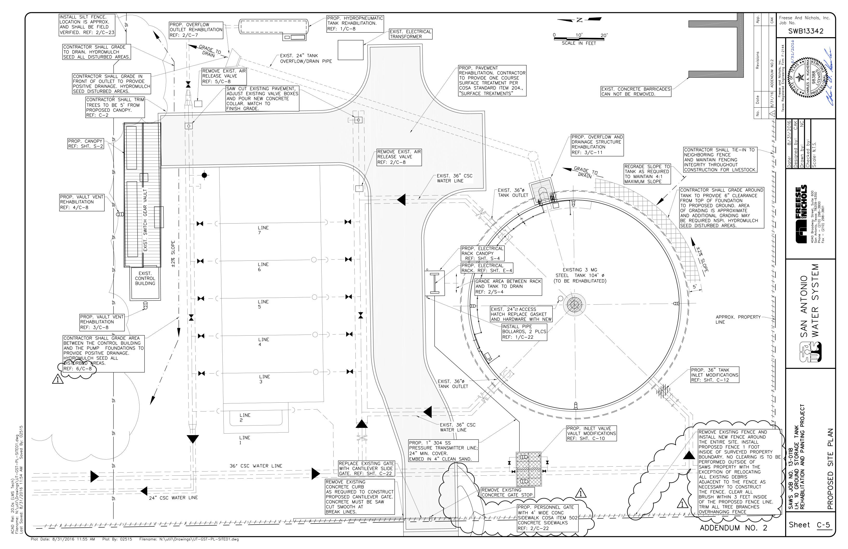
REPLACE EXISTING J-BOXES, PRESSURE SWITCHES AND ABOVE GRADE CONDUITS AT PUMP SUCTION, AS SPECIFIED, 4-PLCS. SEE DETAIL 3
